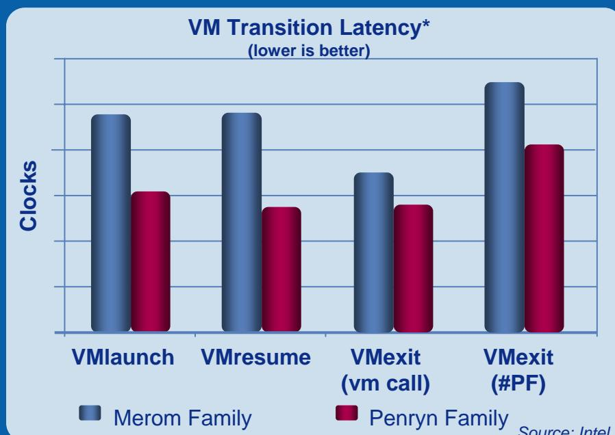
\* Comparisons based on RTL simulations via micro-kernel workloads with cache hits
