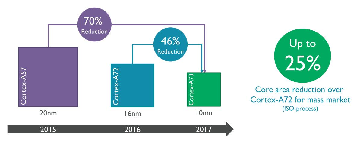
Cortex-A73 reduces footprint allowing additional silicon area for other IP
